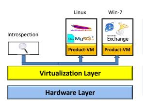
Using a trusted, dedicated virtualization layer program to monitor the running VMs
