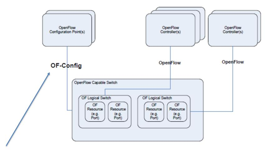
OF-CONFIG uses NETCONF protocol as its transport (implies SSH/TLS)
